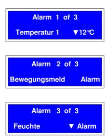
The maximum number of alarm messages is displayed in the top line. The meaning of the icon prefixed to the measured values is the same as that used for the "Values" display (also refer the Values Submenu section).
