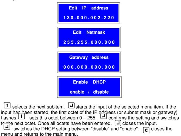
**Warning:** If a network setting has been changed, a reboot of the Processing Unit will be performed in this case and the new network settings will be accepted.
