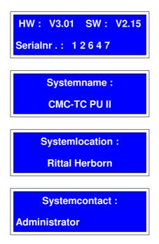
scrolls the display information. The values for "System name", "System location" and "System contact" can be entered from the terminal menu or the web browser.
